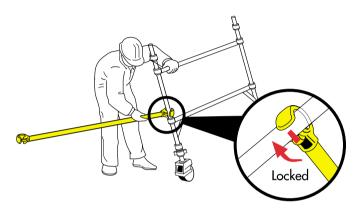
Position the ladder frame as shown and fit the other end of the horizontal brace onto the vertical, just above the bottom rung. Fit a second horizontal brace between the bottom rungs on the other side of the frames to square the tower.
