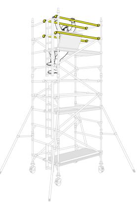
Continue until the required height is reached. Reposition the fixed deck to the required platform height and fit a trapdoor deck alongside it as shown in **stage 7**. Fit a single diagonal at the top of the tower as shown in stage 7. Fit the final guardrails as shown in stage 7.
